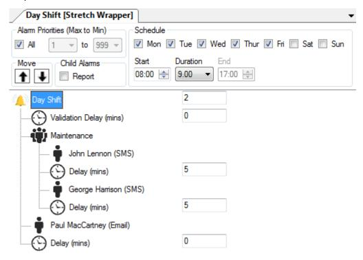
When an alarm occurs in an area, alarm plans are started if the alarm conditions meet the criteria set in the plans.
